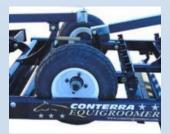
Tires are located inside the frame for optimal gooming coverage.
